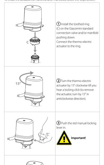
4 Electrically connect the actuator according to the electrical diagrams.
