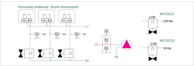
**R473M** thermo-electric actuators equipped with a stroke-end micro switch enable to easily activate circulators or zone valves. They are generally connected to ambient thermostats taking into consideration that the R473M is closed when there is no voltage (while the micro switch is electrically open in such status). To control significant power loads, we recommend installing a relay to prevent overloading of the actuator micro switches.
