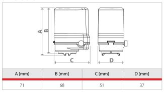
THERMO-ELECTRIC ACTUATORS NORMALLY CLOSED R473, R473M
